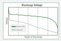
Discover Lithium batteries have a flat and stable discharge curve, which can not be monitored accurately by a voltage-based SOC indicator. For accurate fuel gauge and SoC, a Discover Battery Discharge Indicator is necessary.
