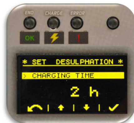
09D The mask on the side shows what appears by selecting the word "Charging Time"
