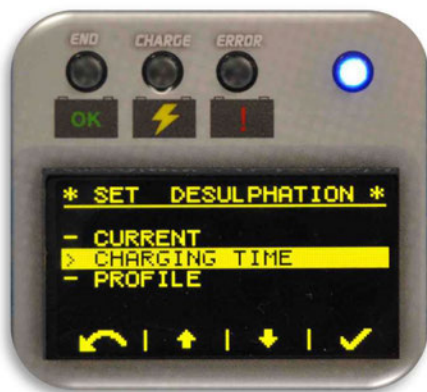
09D The mask on the side shows what appears by selecting the word "Charging Time"
